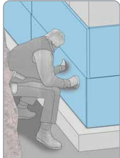
Use of insulating panels below ground.
